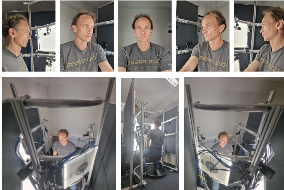
16 synchronized 12MP, 30fps cameras
